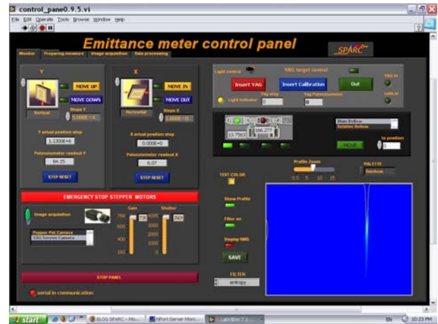
Figure 5. Control Panel for remote control of motors and actuators and digital camera.
