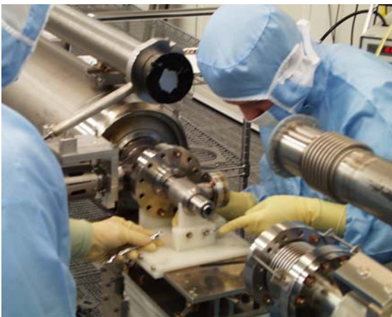
Fig.A.4.4: Installation of a beam pipe short side fixture for dismounting of a flange
