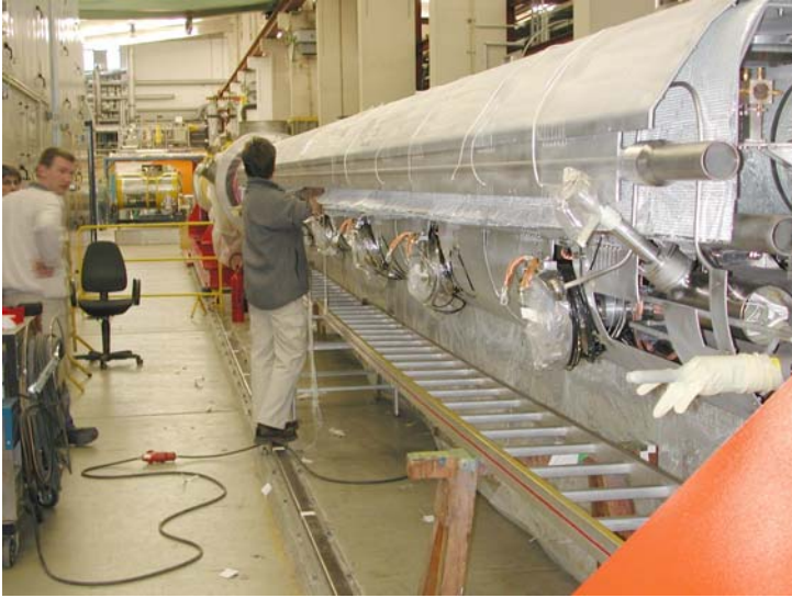
Fig. A.5.7: Mounting of MLI at the 5-K shield
