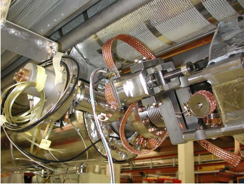
Fig.A.5.3: Tuner parts and main coupler parts at the inter-connection of two cavities at the cavity string
