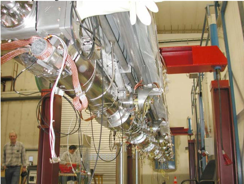
Fig.A.5.3: Tuner parts and main coupler parts at the inter-connection of two cavities at the cavity string
