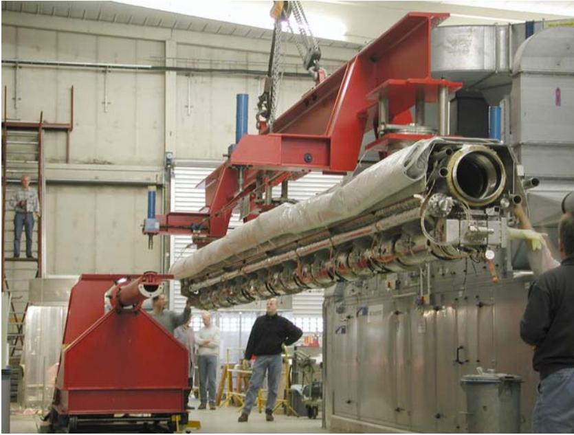
Fig. A.5.5 : Transport of the cold-mass and cavity-string to the cantilever
