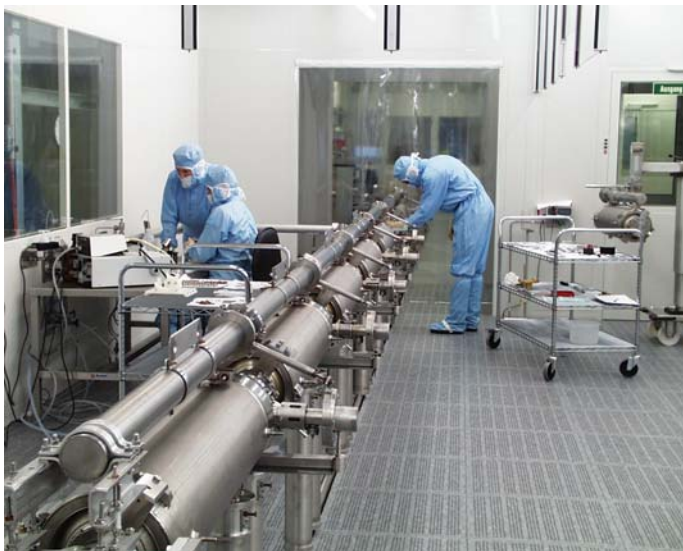
Fig. A.4.1: A complete cavity-string in the clean room
