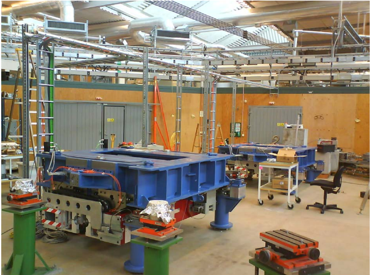
Fig. The two undulators and chicane (hidden in between) in place in the MAX-lab hall.
