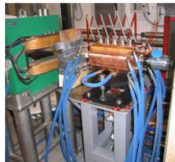
Figure 6: RF deflector installed in SPARC.
