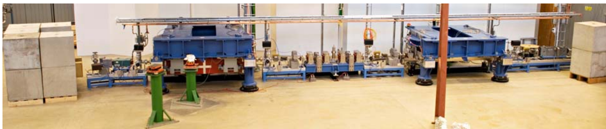
Fig 1. The beamline at MAX-lab with the two undulators of the optical klystron and the chicane in the middle. In the background the laser hutch for the seed laser system.
