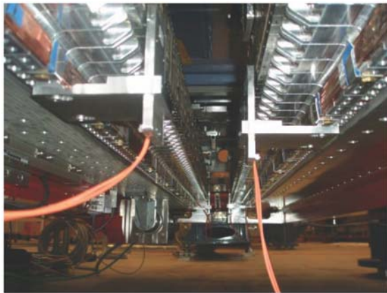
Fig 28. Radiator of the APPLE II type in operating position without vacuum chamber. Four power meter sensors (see below) at each undulator end (orange cable) are installed.
