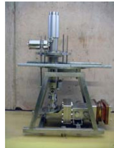
Figure 2: TTF-III coupler mounted on the test stand
